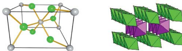
Figure 2. Sketch of the rutile structure of \text{MgF}_2 (left) and the octahedral arrangement in the 3D structure (right). The 3D structure can be rationalized by chains of edge-bridged \text{MgF}_6 octahedra that are corner-bridged to an adjacent chain.
